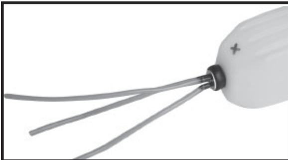
Blow through one of the lines to ensure the fuel lines have not become kinked inside the fuel tank compartment. Air should flow through easily.
