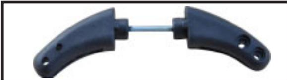
Control horn of Rudder.
