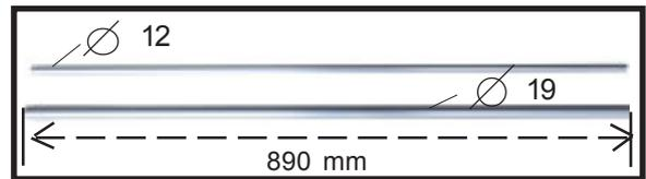
\*\*\* Test fit the aluminium tube dihedral brace into each wing haft. The brace should slide in easily. If not, use 220 grit sand around the edges and ends of the brace until it fits properly.
